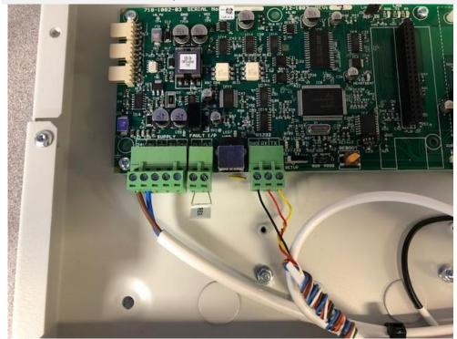
Note the setup switch position on the picture MXP-510 BMS to ESP.
